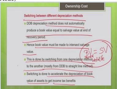
So, another important factor which we are going to discuss today is about switching between different depreciation methods, this is very important as I told you, DDB stands for double declining balance the depreciation method, so, DDB method does not automatically produce a book value equal to the salvage value at the end of the recovery period many cases you can see that the estimated book value can go below the salvage value.
