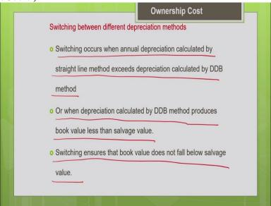
So, switching occurs when the as we discussed just now switching occurs when the annual depreciation calculated by the straight line method exceeds the depreciation calculated with a DDB method it occurs as the initial stage of DDB may be higher than the straight line method as the age
