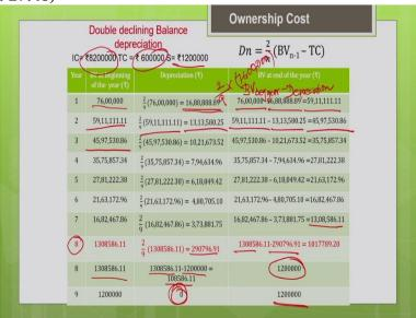
Now, let us move on to the double declining balance method. In double declining balance method it is totally different from the earlier method as I told you here, we are not using salvage value in the estimation of the depreciation of the machine. So, you are going to depreciate the instantaneous book value. So, for the first year, what is the book value at the beginning of the year? It is 76 lakh how did you get this up to 76 lakh your initial cost is 82 lakhs minus your tire cost 6 lakh.
