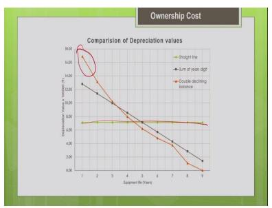
This is just a graphical representation of the depreciation values estimated by 3 different methods you can see straight line method is always constant double declining method this one is giving you the accelerated depreciation more depreciation in the early age of the life of the machine.
